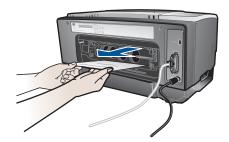
**c** If the jam is not there, push the latch on the top of the auto-duplex unit and lower its cover. If the jam is inside, carefully remove it. Close the cover.
